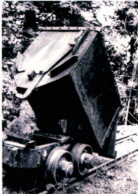
Figure 9. Ore cart on tracks in Kittitas County. Its position shows how rock would be unloaded through hinged door. Ellensburg Public Library Photographs, Identifier MNG-035.
