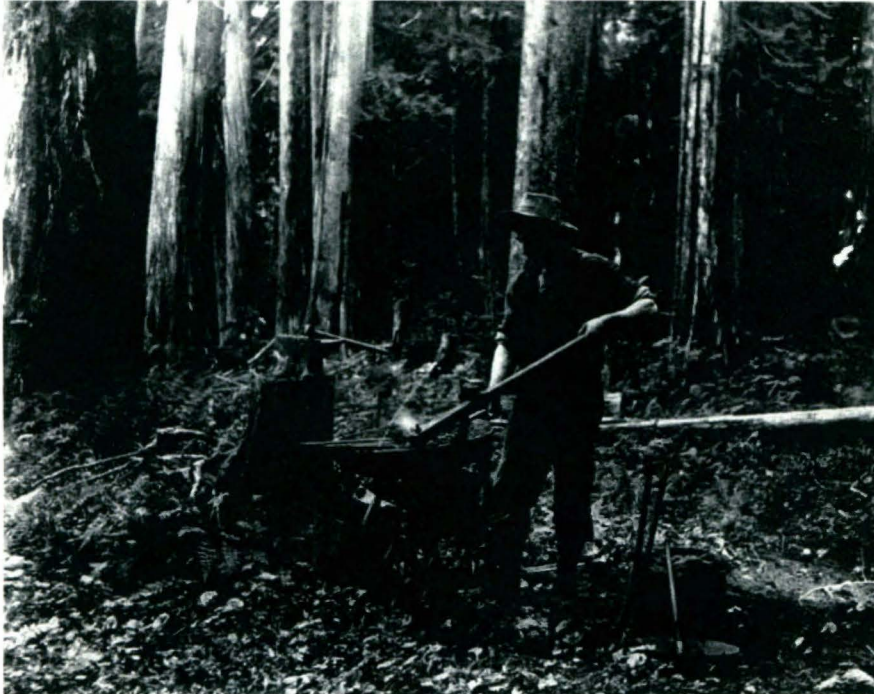
Figure 10. A hard rock miner and makeshift blacksmith shop near Snoqualmie Pass in 1899. The "ducks nest" was a small portable forge and clay pot that was used in many remote mining camps. University of Washington Special Collections, Repository Collection 548.
