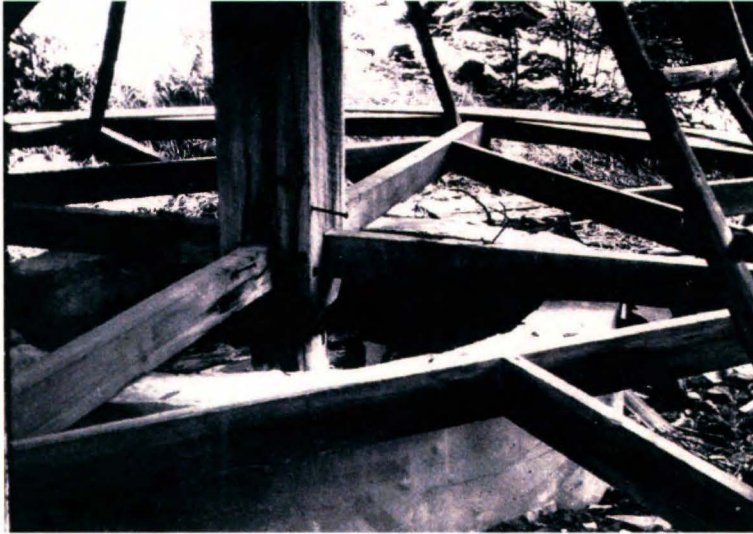
Figure 13. Arrastra with base made of concrete located in the Swauk Mining District. Large stones or steel balls would be dragged or rolled in a circular motion around the inside perimeter of the base. Ellensburg Public Library Photographs, Identifier MNG-034.
