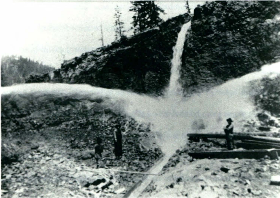
Figure 5. Hydraulic mining operation in the Swauk Mining District ca. 1910. Central Washington University Archives, Identifier MS002-06-02.
